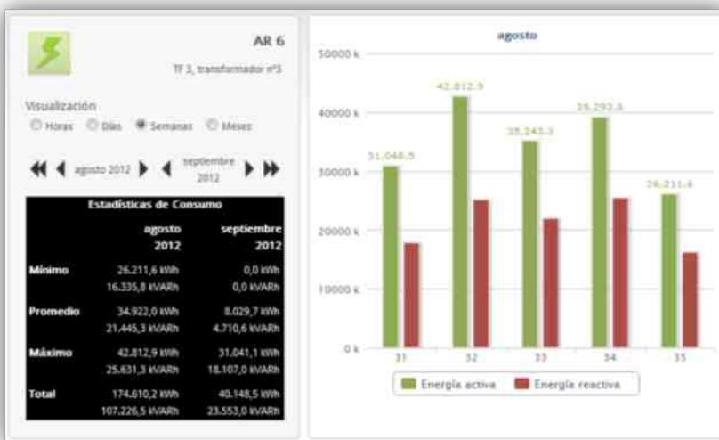
\*\* In this others panels shows measurements recorded as curves and bars with different measurement periods: hours, days, weeks and months.
